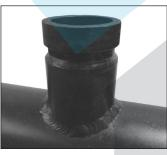
2. CHECK GROOVED END OF SPRINKLER PIPING: The outside surface of the sprinkler piping, between the groove and the end of the sprinkler piping, shall be generally free from indentations, projections, weld seam anomalies, and roll marks to ensure a leaktight seal. All oil, grease, loose paint, dirt, and cutting particles shall be removed.
