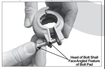
7. INSTALL BOLT: Install the bolt through the housings. Verify that the head of the bolt faces the angled feature of the bolt pad, as shown above.
