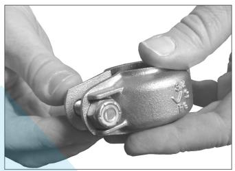
8. INSTALL NUT: Thread the bolt into the nut until the top of the nut is flush with the end of the bolt, as shown above. Verify that the gasket remains seated in the gasket pocket of the housings and that the nut is engaged with the flat features of the bolt pad.
