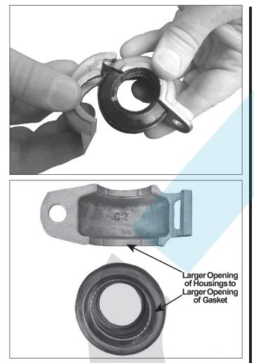
6. REASSEMBLE STYLE V9: Place the lubricated gasket inside the gasket pocket of one Style V9 housing. NOTE: For all sizes other than the 1-inch x 1-inch/33.7-mm x 33.7-mm, verify that the larger opening of the gasket is facing the larger opening of the housings, as shown above. Engage the tab of the one housing with the slot of the other housing, and close the housings around the gasket.
