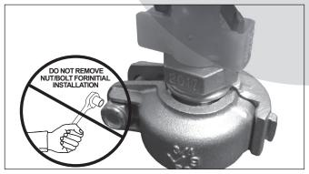
1. DO NOT DISASSEMBLE THE STYLE V9: The Style V9 is designed so that the installer does not need to remove the bolt and nut for installation. This facilitates installation by allowing the installer to directly install the Style V9 onto the sprinkler piping's grooved end.
