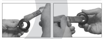
5. LUBRICATE GASKET: Apply a thin coat of Victaulic Lubricant or silicone lubricant to the gasket sealing lips and exterior. NOTE: It is normal for the gasket surface to have a hazy white appearance after it has been in service.
